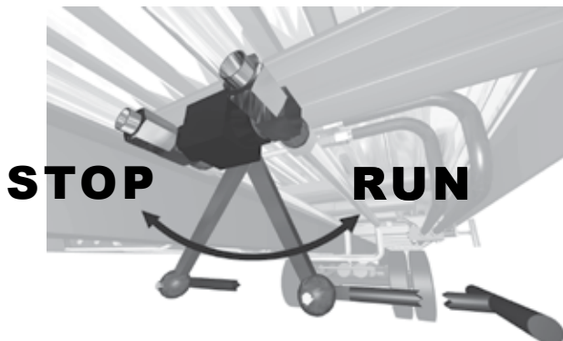
PULL TO UNLOAD Handle Pulled Completely Out
